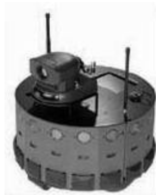
Figure 4: The Magellan Pro mobile robot, it has 51 sensors: 16 ultrasonic sonars, 16 infrared distance sensors, 16 bumpers, 2 wheel encoders and a colour camera.
