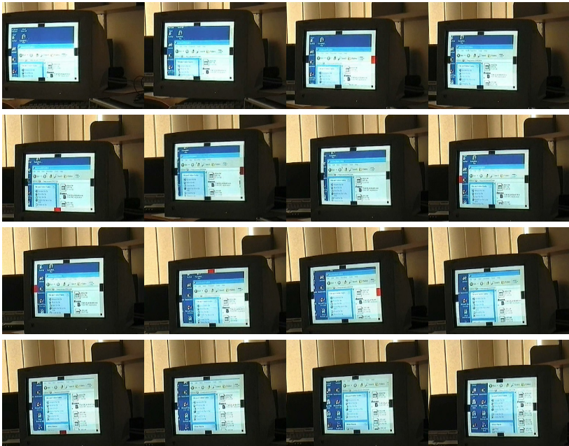
Fig. 2. Snapshots (ordered from left to right and from top to bottom) taken every 20 frames (800ms) from a video recording of our BCI mouse in action. The user wanted to scroll down.
