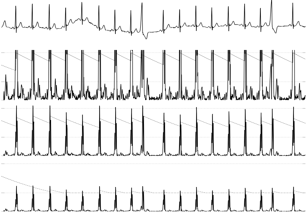
Fig. 1. A tract of ECG signal from record 116 (upper panel) and the output produced by the quasi-linear filter with consecutive samples along with the behavior of the threshold (dashed line) on (top to bottom) the original signal, amplitude reduced by a factor of 5, amplitude reduced by a factor of 10. The lower panels also include two dotted lines which represent the extrema Y_{max} and Y_{min} for the threshold.
