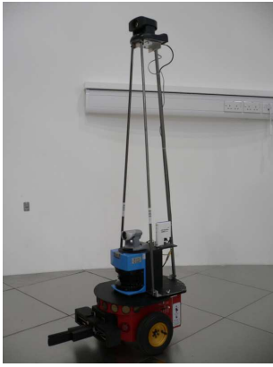
Fig. 4. Robot equipped with laser and PTZ camera for the experiments. The camera used is the black one on the top, about 1.5m high. The blue device is the laser, at approximately 0.4m from the floor.
