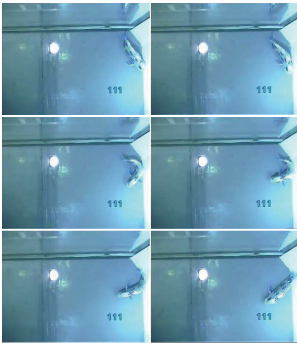
Fig. 19 Video Sequence of blue G9 C-shape sharp turn, time step between two neighbour clips is 0.5 s. The order of video sequence is from left to right and from top to bottom.
