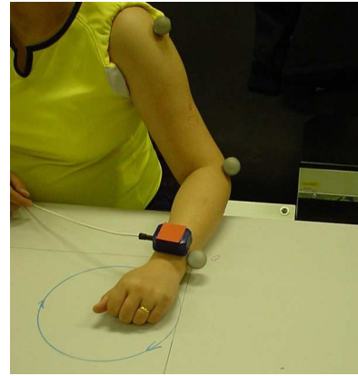
Fig. 5. Subject wearing both an inertial sensor and three ball markers, performing a circle motion.
